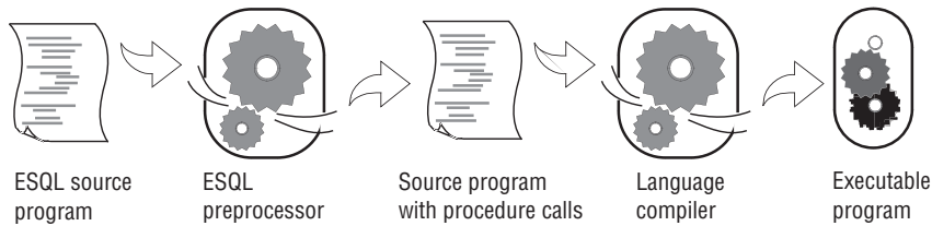
Figure 8-1. Overview of Processing a Program with Embedded SQL Statements
