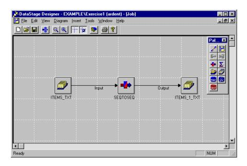
On the left side of the window is a Sequential File stage labelled ITEMS\_TXT, and on the right side of the window is another Sequential File stage, labelled ITEMS\_1\_TXT.
