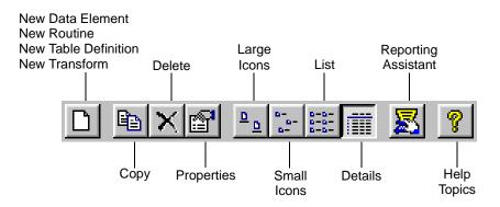
You can display ToolTips for the toolbar by letting the cursor rest on a button in the toolbar.
