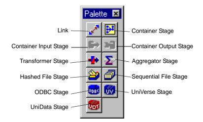
By default, the tool palette appears in the DataStage Designer window, but you can move it anywhere on the screen. To display ToolTips, let the cursor rest on a button in the tool palette.
